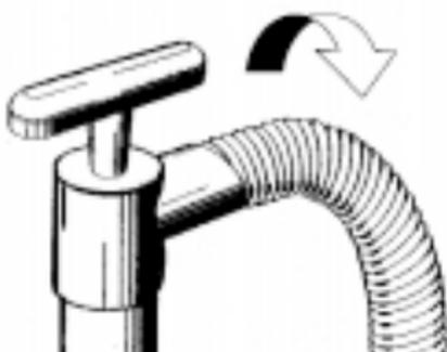
Rotate your right hand back toward you to turn the hose into the thread. Turn the hose into the sleeve until it stops. Give the hose a strong pull with your right hand to make sure that the hose is properly seated into the threaded sleeve.
